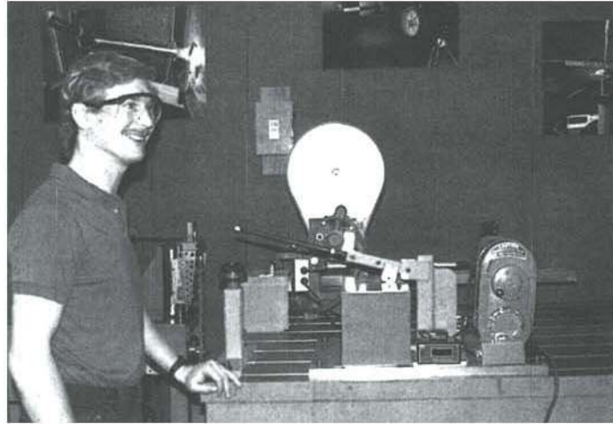
Easton Ahead sticks were created by drummer/engineer Rick Grossman. Tests were performed on machines like this one: the world's only drumstick-playing robot.
